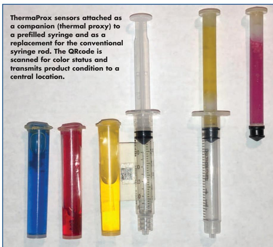
**ThermaProx sensors attached as a companion (thermal proxy) to a prefilled syringe and as a replacement for the conventional syringe rod. The QRcode is scanned for color status and transmits product condition to a central location.**
