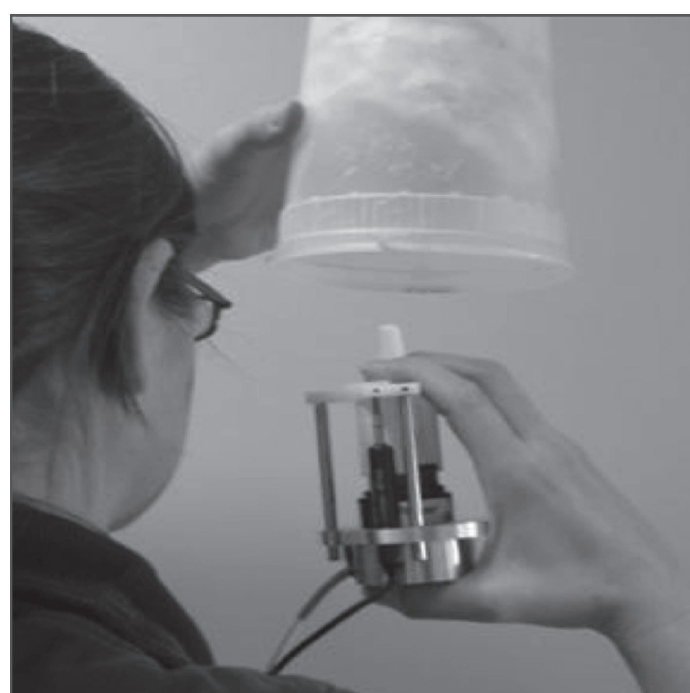
Figure 1. Hand Actuation Monitor, (HAM, InnovaSystems) which was used to Capture Actuation Parameters
